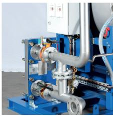
Seawater desalination plants are used, among other places, on cruise ships, to produce drinking and operating water. HEROSE safety valves are produced in seawater-resistant bronze and can therefore be used for a wide variety of applications.
