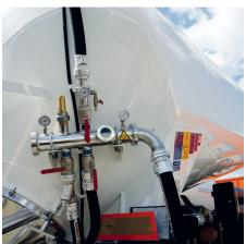
In Europe, silo trailers for the transportation of powdery and granular goods are highly successful. One of the reasons for this success is the HEROSE safety valve for securing the pneumatic discharge. Thanks to its robustness, the valve also operates perfectly under extreme conditions of use.
