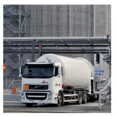
Special road trailer are used to transport LNG from the liquid gas storage facility to the users' satellite stations. Because of frequent filling, transportation and unloading, they are subjected to extreme stresses. HEROSE supplies the valves for liquefied natural gas, approved for LNG according to DIN EN 12567.
