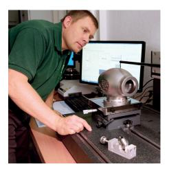
With a contour measuring device, even dimensions which are difficult to access can be checked.
