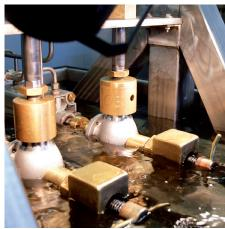
100% leak tests of mechanically machined body at the nominal pressure.
