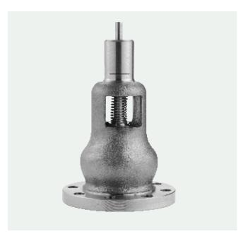
Ramén type VAC100 is a vacuum valve for protection of pressure vessels, tanks, containers, silos, hoppers, piping and other designs that may be exposed to under pressure (by media, cleaning processes, thermal variations, etc). The VAC100 will open automatically when the pressure of gases or vapors goes below 0,85-0,9 bar(a) (can be ordered with other set pressure on request) giving the construction a robust and trusted protection against vacuum that can cause unrepairable damage to any system.
