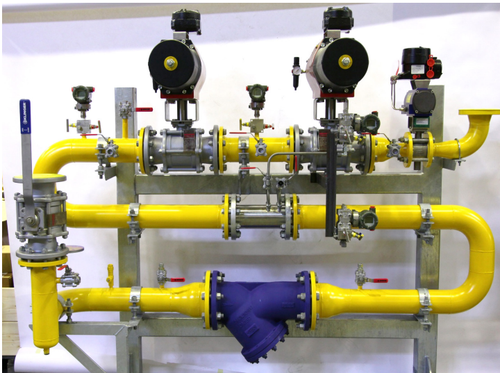
Ramén ball sector control Valve on a valve station upstream burner
