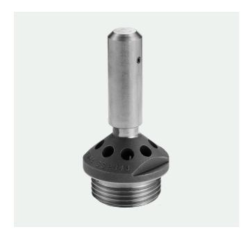
The Ramén type VAC112 is a vacuum breaker made in stainless steel. The VAC112 is used to protect pipelines and closed containers in steam or fluid system for pressures up to 64 barg.
