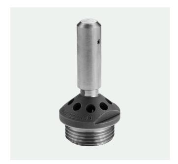
The Engelsberg type VAC112 is a vacuum breaker made in stainless steel. The VAC112 is used to protect pipelines and closed containers in steam or fluid system for pressures up to 64 barg.
