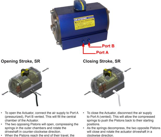
When the Pistons reach the end of their travel, the actuator driveshaft will be in the closed position.
