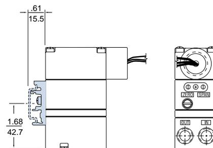
DIN Rail Kit suitable for EN-50035, EN-50045 and EN-50022 Rails
